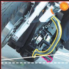
*Every Paladin Highway Bar is checked on its motorcycle for proper cornering clearance.*
