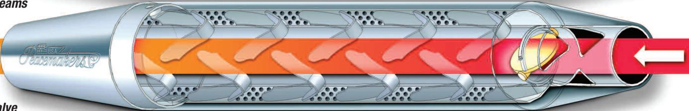
When the Diverter Valves are opened, the exhaust gases also flow through the straight pipe down the center of the muffler, resulting in increased exhaust sound volume and improved engine performance.
