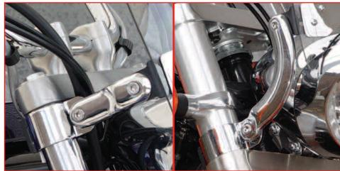
The Flyscreen's Linking Arm mounting hardware is custom designed to fit your individual motorcycle.
