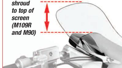
**3** Measured from top of stock headlight shroud to top of windscreen (see diagram above)
