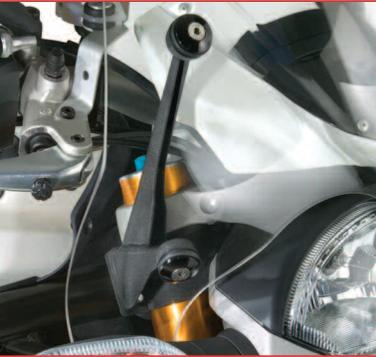
The Monster's clamps are strong, light-weight, and easy to install. The arms are designed to afford maximum stiffness and minimum weight without any compromise in structural integrity. Black wrinkle finish powdercoat matches the texture of the OEM lower triple clamps.
