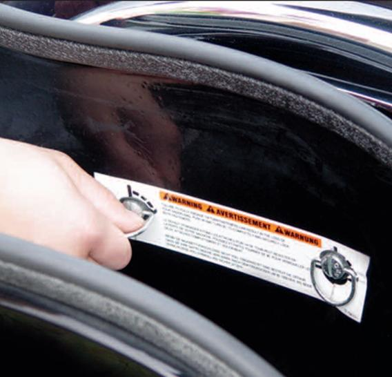
*A quick-detach quarter-turn fastener is located securely inside the bag for “no-tool” quick removal of the saddlebags from the frame.*
