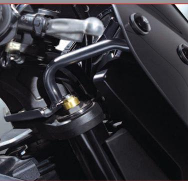
The one-piece B-King mounting system is attached between the risers and the top triple clamp for maximum strength. The black powdercoated finish matches the OEM hardware. Combined with a rubber grommet suspension to the screen, this VStream is an outstanding performer.
